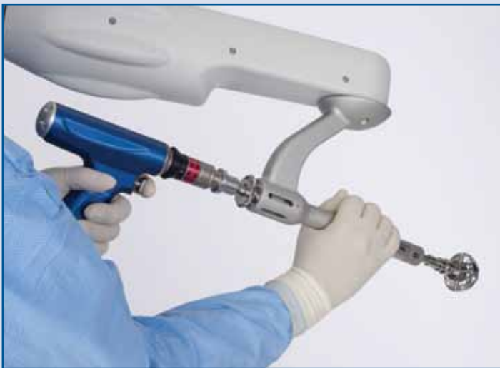
This image demonstrates the use of the robotic arm for proper alignment of the hip socket.
